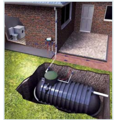
Figure 51: Example of an underground water tank in relationship with the building (Source: https://handymantips.org/about-underground-water-tanks/ )
